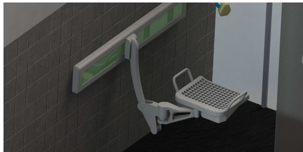
Figure 6. The CAD model of the first prototype of the motorized chair.
