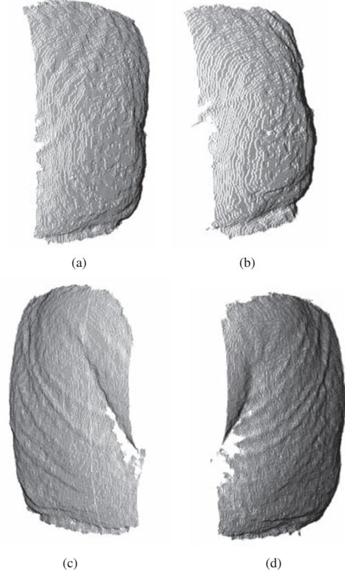
Fig. 4: Point-Cloud representation of the back of the seated subject. (a) Subject is seated with its back straight. (b) Subject is seated with its back bending forward. (c) Subject twists its back right (occlusion of the right arm in the field of view). (d) Subject twists its back left (occlusion of the left arm in the field of view).
