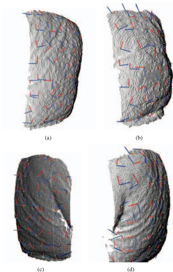
Fig. 5: Point-Cloud representation of the back of the seated subject with one resolution level of local geometric attributes overlaid on the data, for the same subject configurations (a) to (d) depicted in Fig. 4. (a) Subject is seated with its back straight. (b) Subject is seated with its back bending forward. (c) Subject twists its back right (occlusion of the right arm in the field of view). (d) Subject twists its back left (occlusion of the left arm in the field of view).
